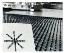
■ Parts cut off will not fall onto sheet metal thanks to part drop system, thus part deformation will be prevented (O)
