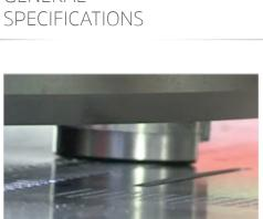
Smooth cutting of sheet metal in requested shape with punch tools up to 88.9 mm In diameter (S)
