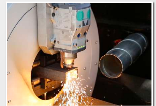
Pipe and profile cutting option allows to cut the pipe, square, rectangular, "U" and "L" shaped profiles.
